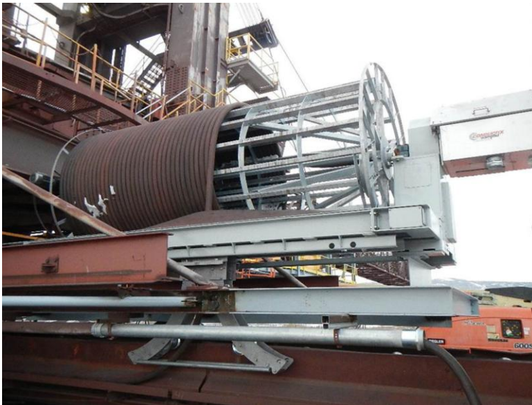
Caption: The new Level Wind Cable Reel accommodates an active travel distance of 1,600 feet (490m) and manages a 4/0 AWG 3 Conductor SHD-GC 5kV All-Temp Industrite cable by Draka (Prysmian Group)
