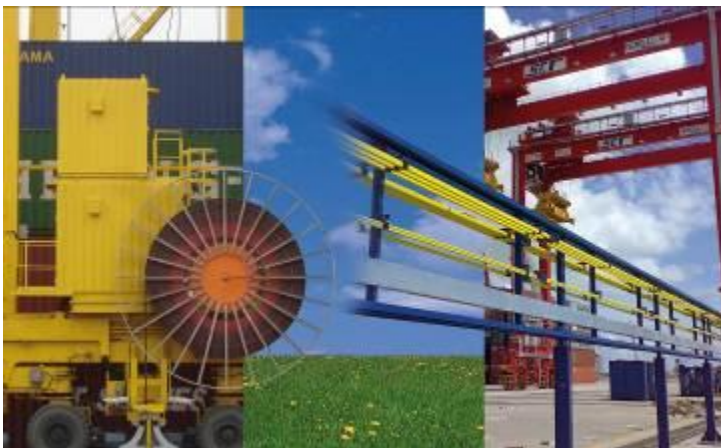
Caption: The electrification of rubber tyred gantry cranes (RTGs) is an approach with an environmentally compatible approach which has already made it possible to save millions of Euros and tons of CO2 around the globe.
