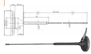
VUA100AH Through insulated remote antenna 419-434 MHz 1/2 wave 0.5 m cable - BNC
