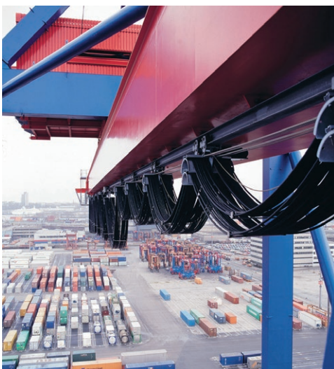
Carrying a heavy load! Motorized cable trolley system program 0380 in combination with program 0375 on a STS-container crane.
